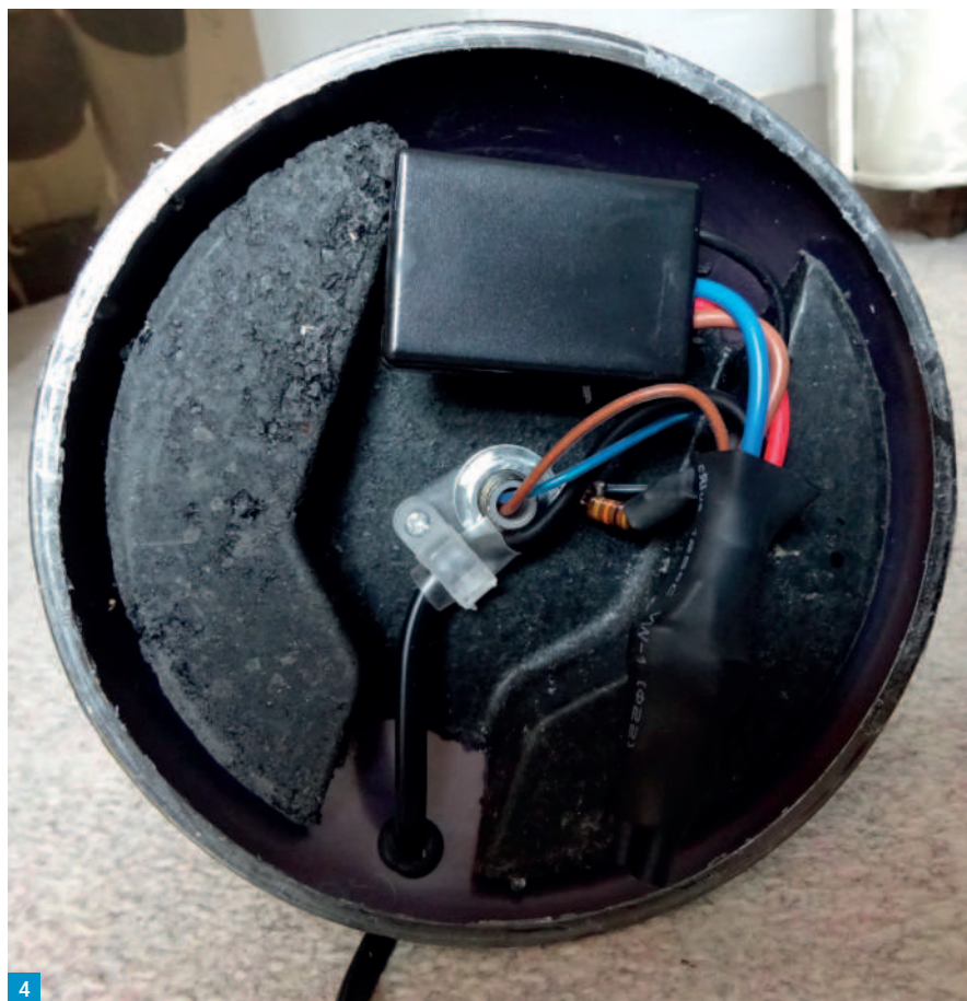
Fig. 1: A high-pass filter – allows UHF TV signals to pass, while attenuating HF and VHF signals.
