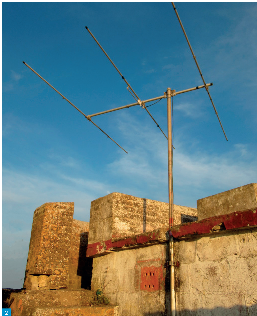
Fig. 2: Kevin ZB2GI's 3 element 6m beam used for his portable operation at the top of the Rock.
