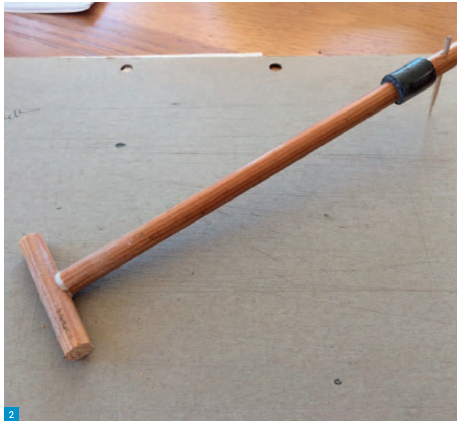
Fig. 1: The kit on arrival. Fig. 2: The author's home-made tool for holding components in place. Fig. 3: The IC after soldering in place. Fig. 4: The finished toroids in place. Fig. 5: The assembly after 3D printing some suitable supports. Fig. 6: 3D printed insulating bar. Fig. 7: VSWR curve for the balun. Fig. 8: The balun boxed up. Fig. 9: Inside the finished ATUBox. Fig. 10: The ATUBox in situ.
